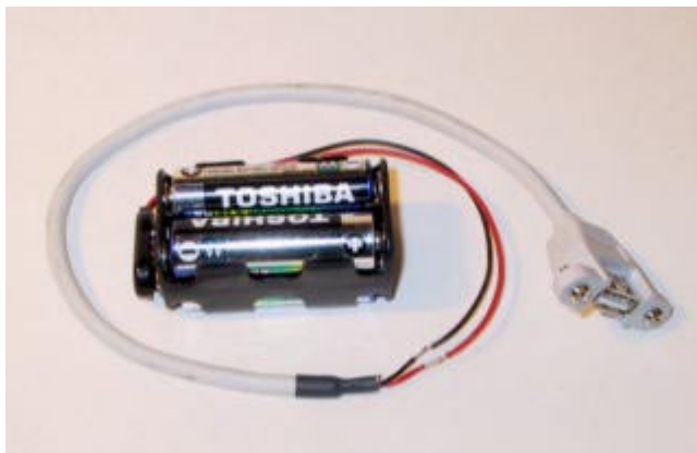
Figure 3 Red Wire to Red Wire, and Black Wire to Black Wire
