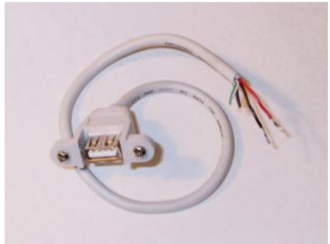
Figure 2 USB Jack Cable, Showing Red and Black wire separated from the others.
